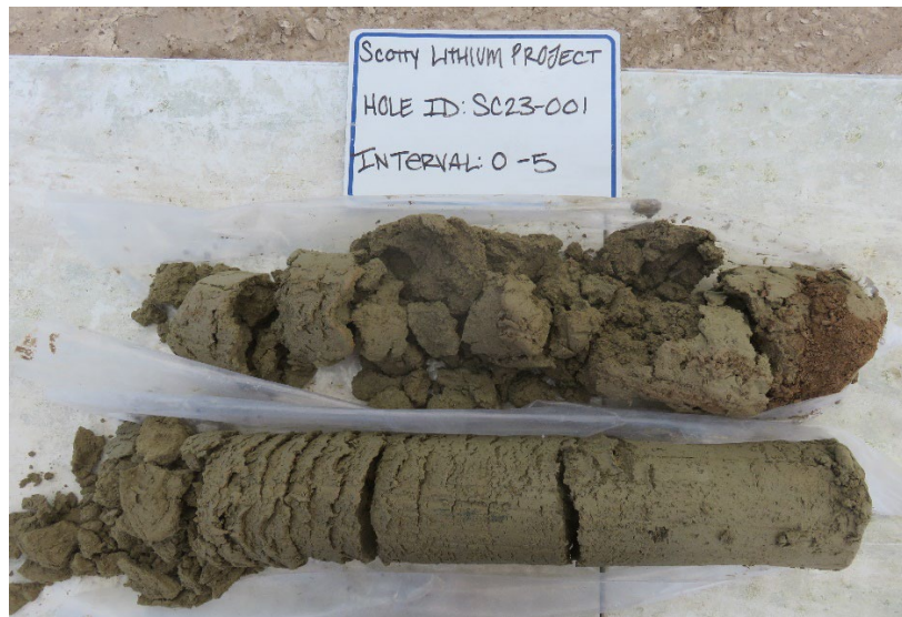
Figure 4-24 Example of Overburdening Sand and Clay at 0.0 - 1.52 m of Hole SC23-001
