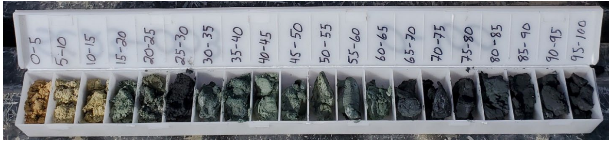
Figure 4-25 Chip Tray from 0.0 - 30.5 M of hole SC23-003 showing brownish red overburdening sediments (0 - 4.75 m), olive green reducing clays (4.75 - 7.62 m, 9.14 - 19.81 m) and blueish green oxidized clays (7.62 - 9.14 m, 19.81 - 30.5 m).
