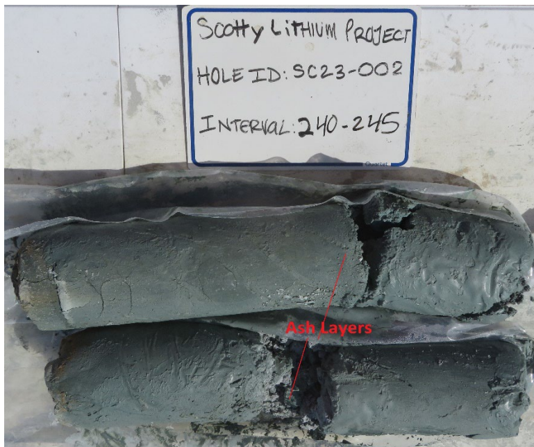
Figure 4-29 Example of Ash Layers From 73.15 m - 74.68 m in Hole SC23-002.
