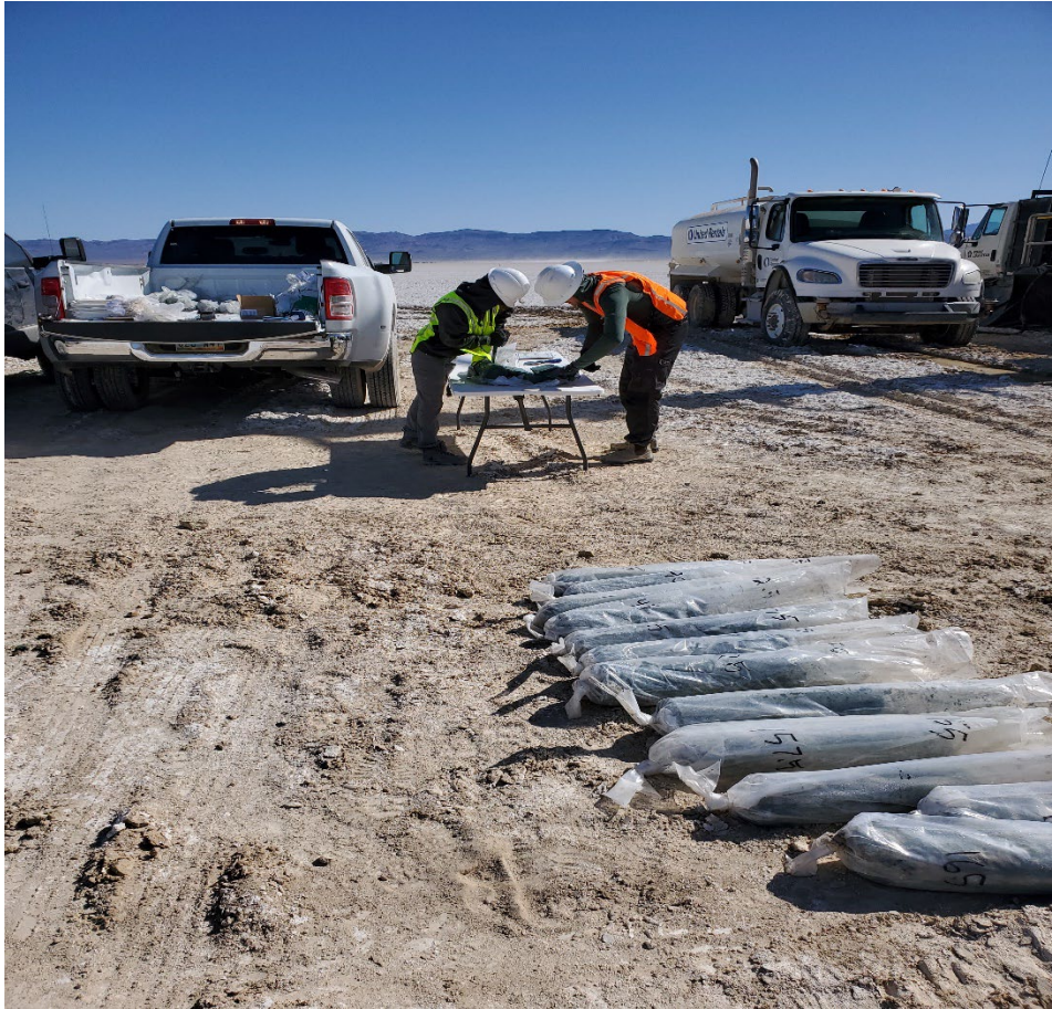
Figure 4-35 2023 Sonic Drill Pad Logging Set Up.
