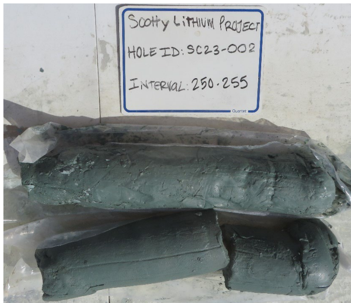
Figure 4-33 Interval 76.2m to 77.72m From SC23-002 Containing 2516 ppm Lithium.
